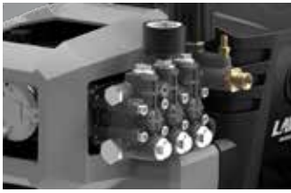
Linear motor pump with stainless steel valves and aluminium head
